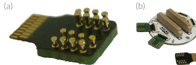
Figure 12: (a) Wire-ZIF-adapter board with loaded wires. (b) Wire-ZIF-adapters connected to a 64-channel EIB.
