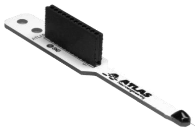
Figure 2: Standard 8-channel probe assembled on a PCB with an Omnetics Micro-series-connector.
