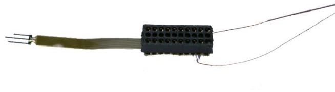
Figure 7: Probe and cable directly soldered to a common strip connector.
